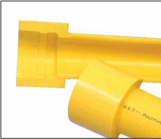
Short Stab Depth Caused by Failure to Use a Depth Gauge
